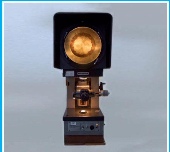
Wall Thickness Measuring Equipment - Profile Projector
