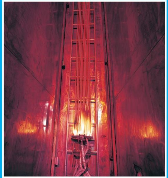
Flame Retardant Test Equipment - IEC 60332-3
