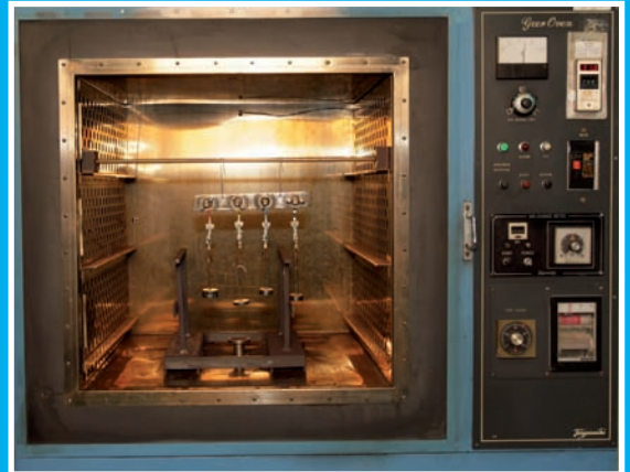
XLPE Hot Set Test Equipment - Oven
