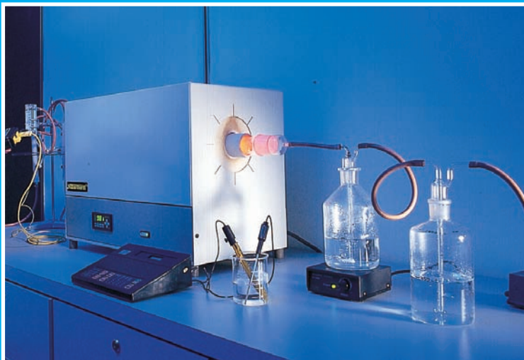
Halogen Content & Corrosivity Tests Equipment - IEC 60754-1 & IEC 60754-2
